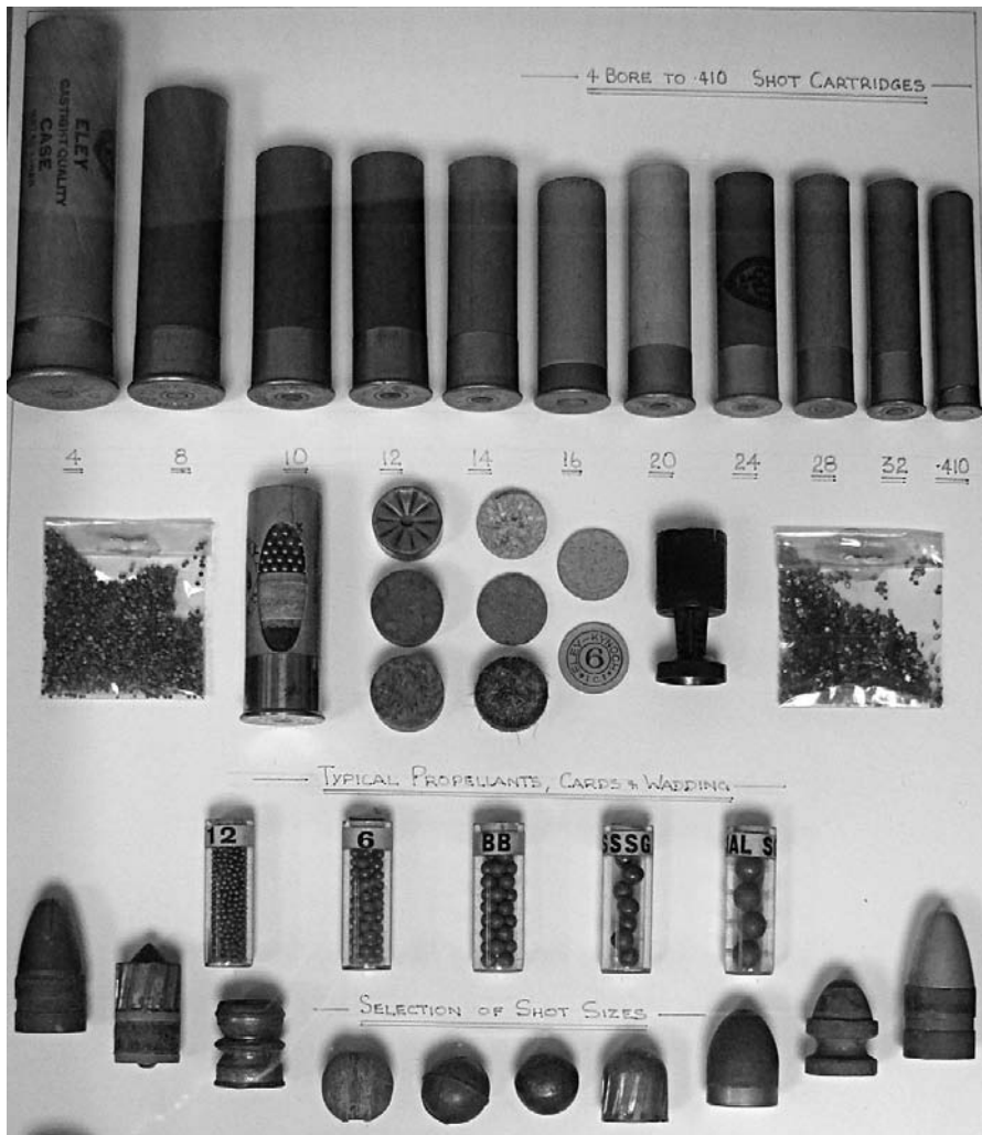
Fig. 15.2 Shotgun cartridges, calibres and missiles. (Photograph reproduced with permission of SPSA Forensic Services.)
