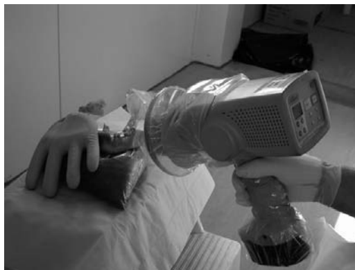
Fig. 17.6 Portable, hand-held X-ray unit in use. (Permission from CIFA.) A colour version of this figure can be found on the book website at www.cambridge.org/9780521705684 .
